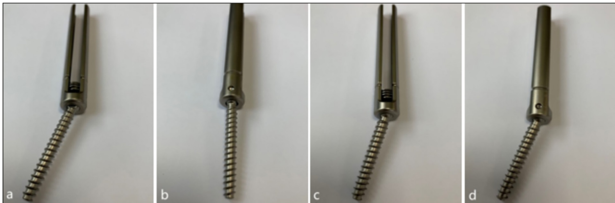
Figure 2. a-b, Due to its unique flat inner core, when the single plane screw is placed in the vertical coronal plane, the screw tail can only move left and right in the horizontal plane and cannot move up and down in the sagittal plane. c-d, The universal screw has spherical inner core, which can swing in both the sagittal plane and the horizontal plane.
