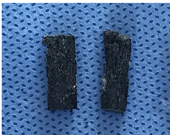
Figure 1. General view of prepared CNTs/PLA/CHI three-dimensional porous scaffolds (0.4 cm* 0.4 cm* 1.5 cm).
