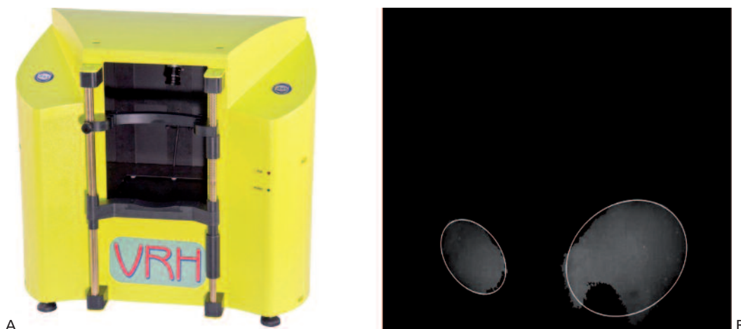
Figure 2. A, VRH instrument; B, elaboration of condensation halos of the airflow of each nostrils on the thermoregulated plate.
