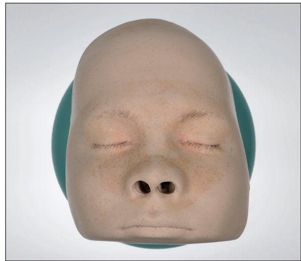
Figure 2. Phantom skull with silicone mask. Phantom with removable silicone mask suitable for photo registration and tactile registration.
