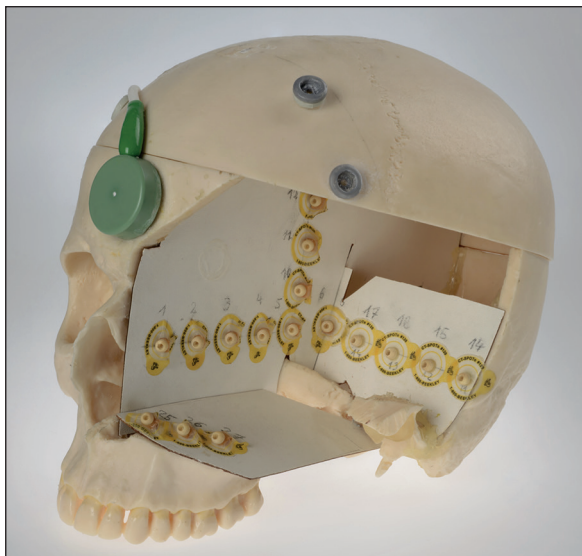
Figure 1. Phantom skull with a total of 27 firmly anchored markers (1-9 in the sagittal, 14-21 in the axial and 10-13 and 22-27 in the coronal plane) and localiser (in green).
