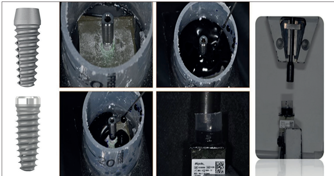
Figure 1. Preparation of the CS and IH implants specimens for the experimental tests. Both groups after submitted to 5 \times 10^4 loads to evaluate the microleakage through toluidine blue infiltration.
